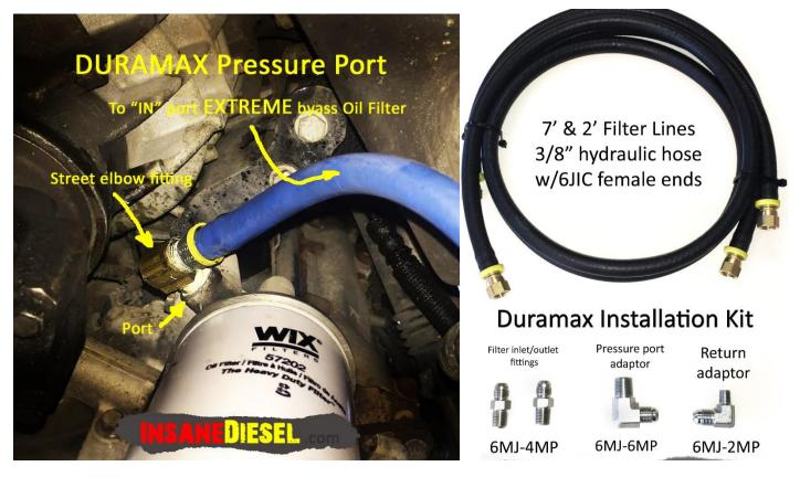
5b) Install street elbow fitting, utilizing thread sealer or Teflon tap, into vacated port on oil filter housing. Aim away from front driveshaft.
